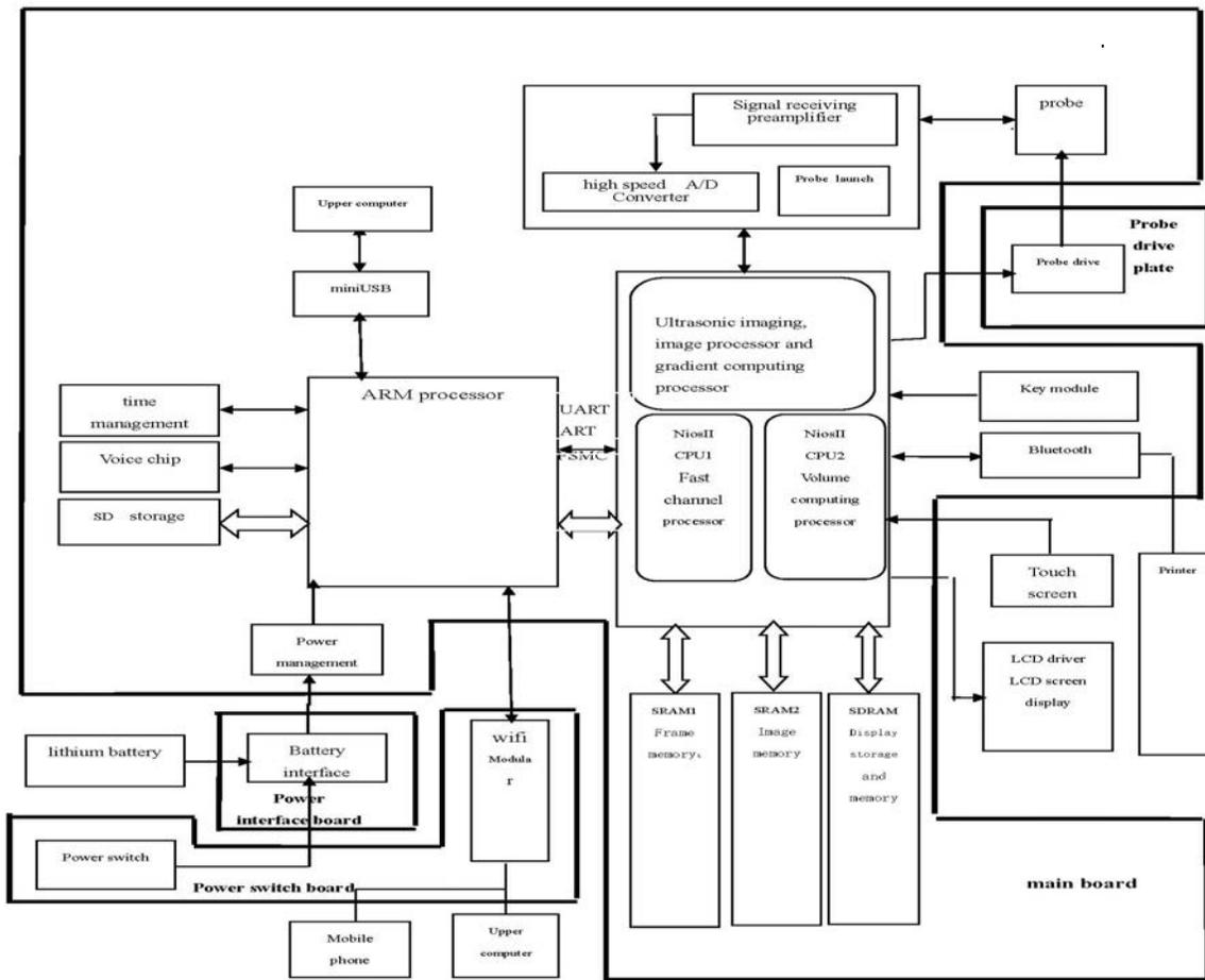
Figure 3-4 Block diagram of electrical principle of M2-W/M2
